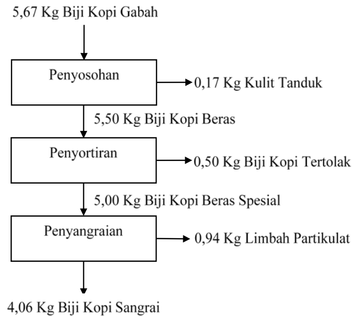
Gambar 12. Diagram Alir blok pengolahan sekunder kopi Figure 12. Block flow diagram of secondary coffee processing
